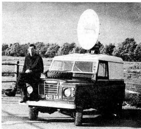
Part of the G3YGF portable 10GHz troposcatter system, showing Land-Rover and roof-mounted 4ft dish
